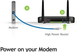
Connect the other end of the cable to the blue Modem port on the High Power Router.
