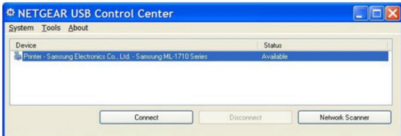
**Step 7:** Click the **Disconnect** button at any time to release the connection. The status then changes to Available.
