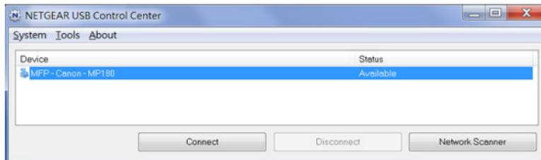
Once the Connect button has been clicked once on all computers in the network, the utility on each of them automatically handles the printing queue and handling. The status of the printer should appear as Available on all of the computers.
