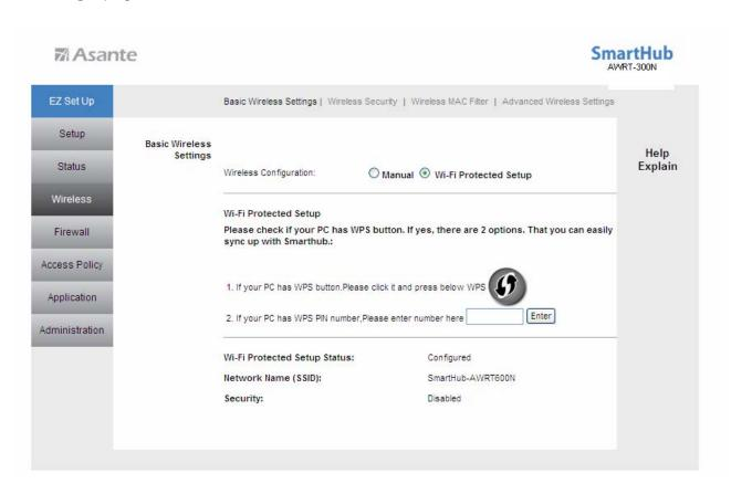
WiFi Protected Setup supports two types of connection: Push Button Configuration (PBC) or Personal Identification Number (PIN).
