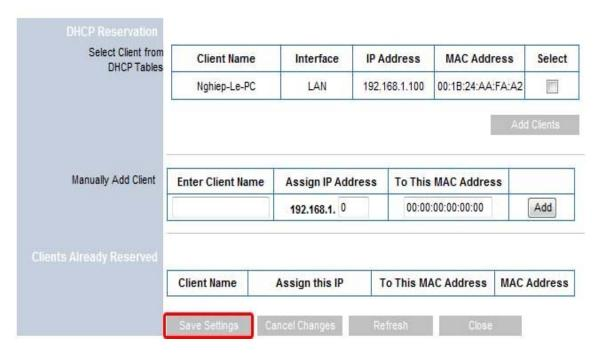
**Step 1** Enter the Static IP Address in the **Assign this IP** field.
