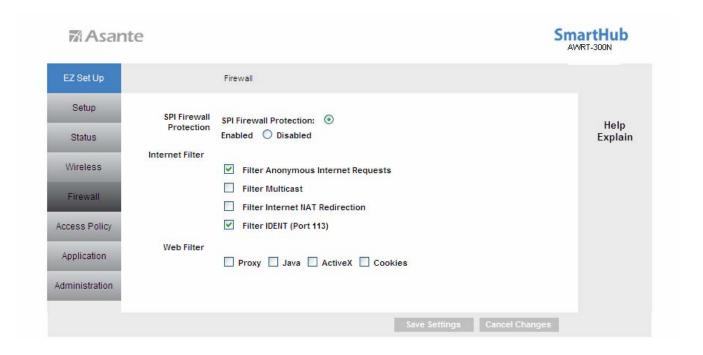
**SPI Firewall Protection**: Select to enable or disable Stateful Packet Inspection. When enabled, access to the router from internet/wan by various protocols like ICMP are denied.
