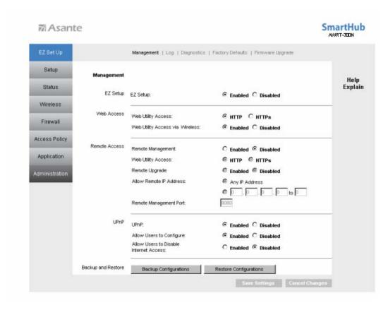
**EZ Setup**: Select to enable or disable **EZ Setup**. If **EZ Setup** is disabled, the user is allowed to access internet whenever he/she is connected to the router. If enabled, the user is required to enter username/password to access the internet.
