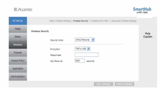
**Encryption**: Select either **TKIP** or **AES** as the encryption method.
