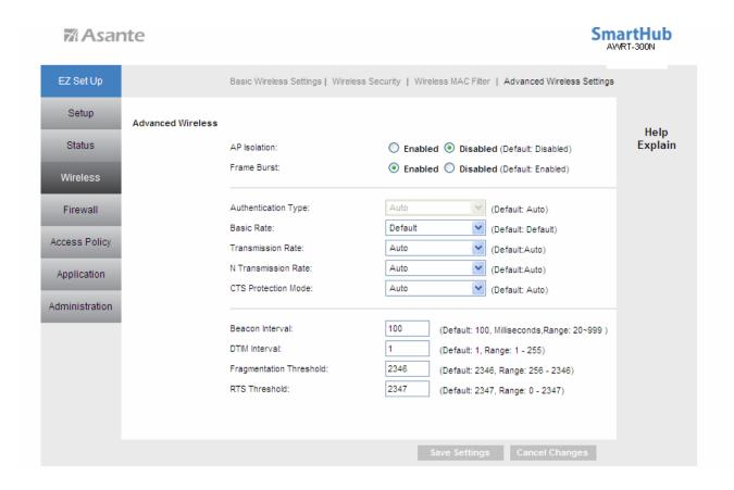
**AP Isolation:** This isolates all wireless clients and wireless devices on your network from each other. Wireless devices will be able to communicate with the Router but not with each other. To use this function, select **Enabled**.
