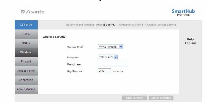
**Encryption**: Select either **TKIP** or **AES** as the encryption method.
