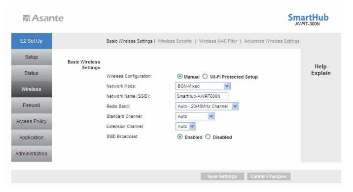
**Network Mode**: If you have 802.11b/g/n 2.4GHz devices on the wireless network, select **BGN-Mixed**. If you have 802.11a/n 5GHz devices on the wireless network, select **AN-Mixed**.
