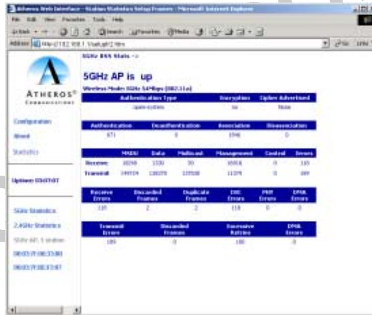
Figure A-15. Basic Service Set Statistics Window for an AP
