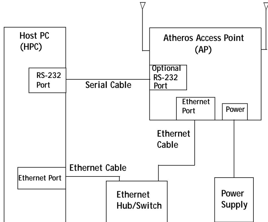
Figure 2-1. Access Point to HPC Connections
