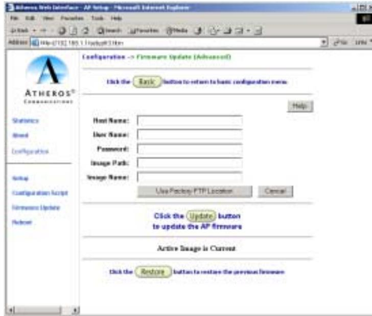
Figure A-14. Advanced Firmware Update Configuration Window
