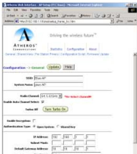
Figure 2-4. System Configuration Window
