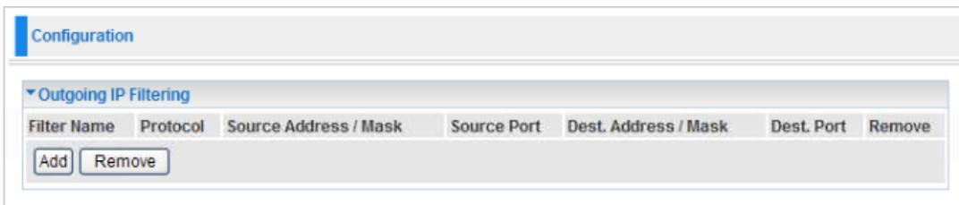
The screenshot shows the 'Configuration' page with a sub-section titled 'Outgoing IP Filtering'. It features a table with columns: Filter Name, Protocol, Source Address / Mask, Source Port, Dest. Address / Mask, Dest. Port, and Remove. Below the table are 'Add' and 'Remove' buttons.
