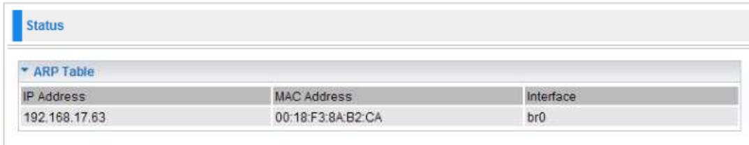
The screenshot shows a web interface with a 'Status' tab. Underneath, there is a section for the 'ARP Table'. It contains a table with three columns: 'IP Address', 'MAC Address', and 'Interface'. The data row shows the IP address 192.168.17.63, the MAC address 00:18:F3:8A:B2:CA, and the interface br0.
