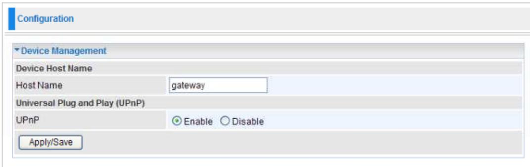
UPnP offers peer-to-peer network connectivity for PCs and other network devices, along with the feature to control data transfer between devices. UPnP offers many advantages for users running NAT routers through UPnP NAT Traversal, and on supported systems. By letting the application control the required settings and removing the need for the user to control the advanced configuration of their device will make tasks such as port forwarding become easier.
