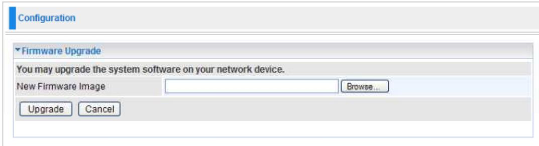
The screenshot shows a web interface for firmware upgrade. At the top, there is a 'Configuration' tab. Below it, the 'Firmware Upgrade' section is expanded. It contains the text: 'You may upgrade the system software on your network device.' Below this text is a 'New Firmware Image' label followed by an empty text input field and a 'Browse...' button. At the bottom of this section are two buttons: 'Upgrade' and 'Cancel'.
