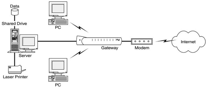
The Intel AnyPoint Networking Gateway 1400 connects directly to a cable modem. Using the gateway and cable modem together enables powerful Internet access on a home or small-business network.
