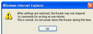
4. A 60-second countdown will appear on the screen. When the countdown reaches zero, the Router's configuration will be restored. The Router's home page should appear automatically. If not, type in the Router's address (default = 192.168.2.1) into the navigation bar of your browser.
