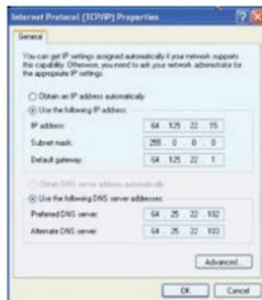
5. If "Use the following IP address" (2) is selected, your Router will need to be set up for a static IP connection type. Write the address information in the table below. You will need to enter this information into the Router.
