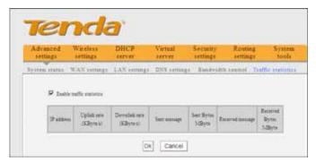
Enable Traffic statistics: It is used to calculate the traffic used by the LAN computers. You can enable it to calculate the traffic for you. Usually, disable it to improve the router's data packet processing ability, and the default is disabled. When this function is enabled, the webpage will refresh automatically every five minutes, meanwhile, each computer's traffic value will refresh automatically.
