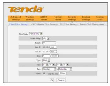
**Example 2** Permit LAN computer with the IP address of 192.168.0.145 to access websites during 8:00 to
