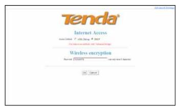
The default access method is ADSL dial-up and the access account and access password are the same as the ADSL dial-up account and password, which you can inquire your broadband ISP. For other access methods, please refer to WAN settings in chapter 4. The wireless password can only consist of 8 characters, the default is 12345678 and you can modify it when necessary.
