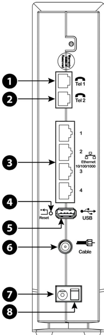
1. Connect one end of the coax cable to the cable outlet or splitter, and the other end to the Telephony Gateway's Cable connector (6). Tighten the connections by hand, then tighten an additional 1/8 turn with a wrench.
