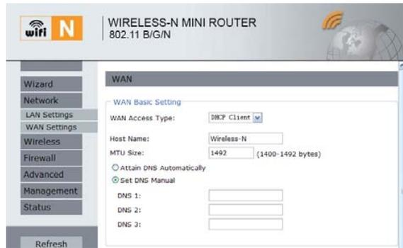
The screenshot shows the WAN Basic Setting page for a Wireless-N Mini Router. The WAN Access Type is set to 'DHCP Client'. The Host Name is 'Wireless-N' and the MTU Size is 1492 bytes. There are three empty input fields for DNS 1, DNS 2, and DNS 3. The 'Set DNS Manual' radio button is selected.
