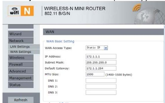
The screenshot shows the WAN Basic Setting page for a Wireless-N Mini Router. The WAN Access Type is set to 'Static IP'. The IP Address is 172.1.1.1, Subnet Mask is 255.255.255.0, and Default Gateway is 172.1.1.254. The MTU Size is 1500 bytes. There are three empty input fields for DNS 1, DNS 2, and DNS 3.
