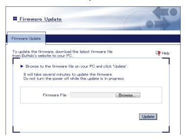
**Note:** Do not turn the power off until update is finished! When the power LED stops blinking and glows steadily, it is safe to turn off the power.
