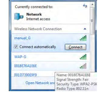
Select the target AirStation and click [Connect]. If you will be connecting to this device in the future, checking [Connect automatically] is recommended.
