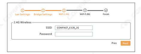
8. Repeater Mode: The AP device can set the internal network segment (the gateway IP should not be the same as the upper device gateway IP). Next, select the name of the wireless SSID signal that you need to relay (distinguish between 5.8GHz and 2.4GHz) and input wireless password.
