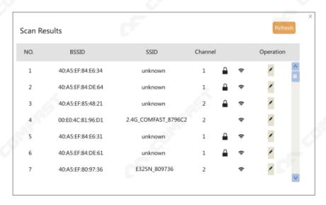
Pls set the SSID and password for the device and click "Next" to finish settings.
