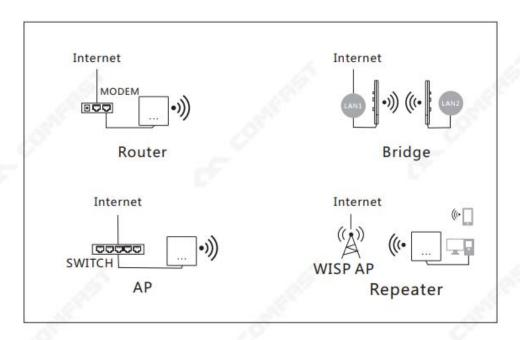
5. Click AP mode and set up IP Address and Subnet Mask. The IP address and Subnet mask should be within the same network segment as upper network and can't be conflict with IP address from upper network router. After settings, you can visit the device from the IP address you have set just now by connecting internet with WAN port of the device or POE adaper LAN port.
