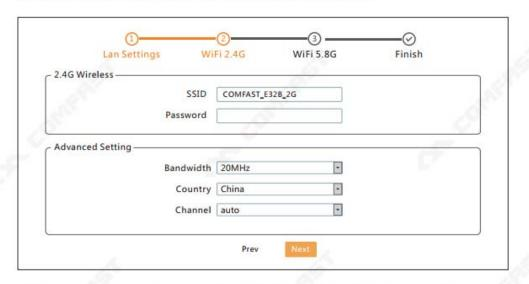
7. Bridge Mode: Pls ensure the WDS in upper network is enabled. AP device can set up intranet segment(do not set the same IP address as the upper router), and then select the wireless SSID signal you need to bridge(Distinguish between 5.8GHz and 2.4GHz) and input wireless password.
