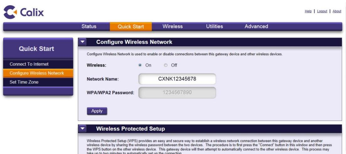
Search the SSID CXNK12345678, type the correct WiFi password, then your Notebook can be connected to the device via WiFi for the internet.
