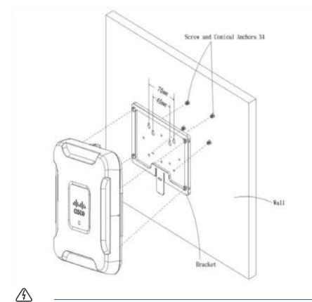
WARNING Insecure mounting might damage the device or cause injury. Cisco is not responsible for damages incurred by insecure wall or ceiling mounting.
