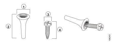
1 7.8 to 8.3 mm/ 2 21.8 to 22.3 mm/ 3 5.5 to 6.0 mm/ 4 17.5 to 18.2mm/ .31 to .33 in .86 to .88 in .22 to .24 in .69 to .72 in
