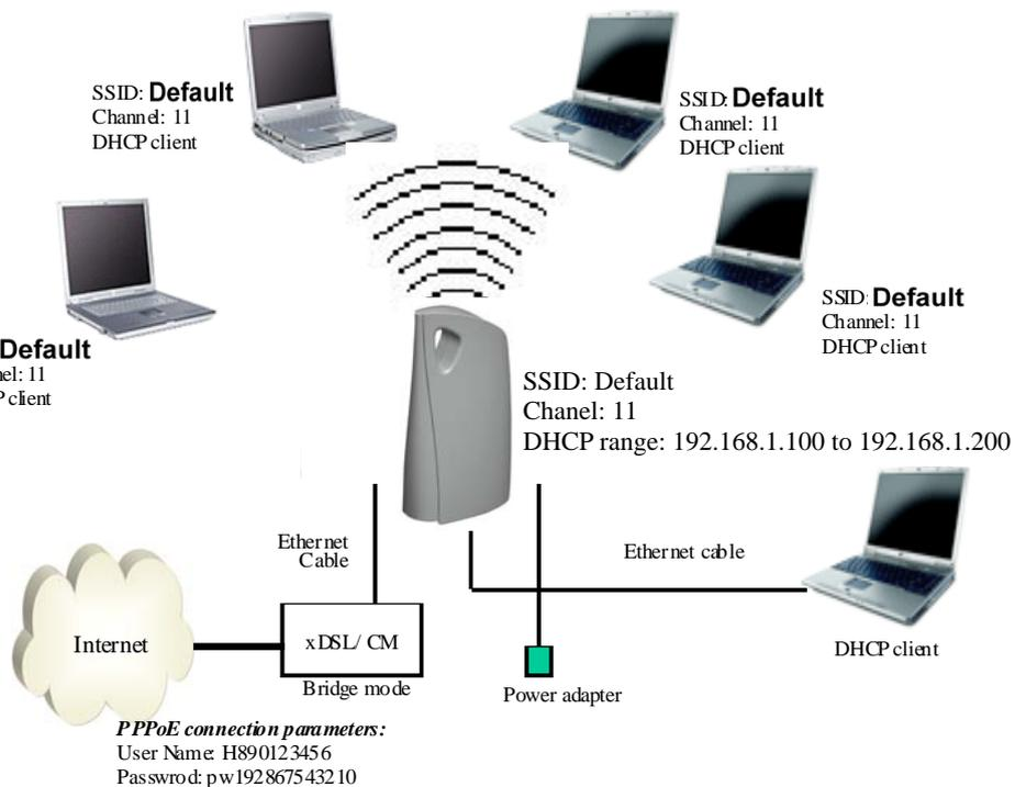
Figure 3 – Configuration Example One – PPPoE on the WAN
