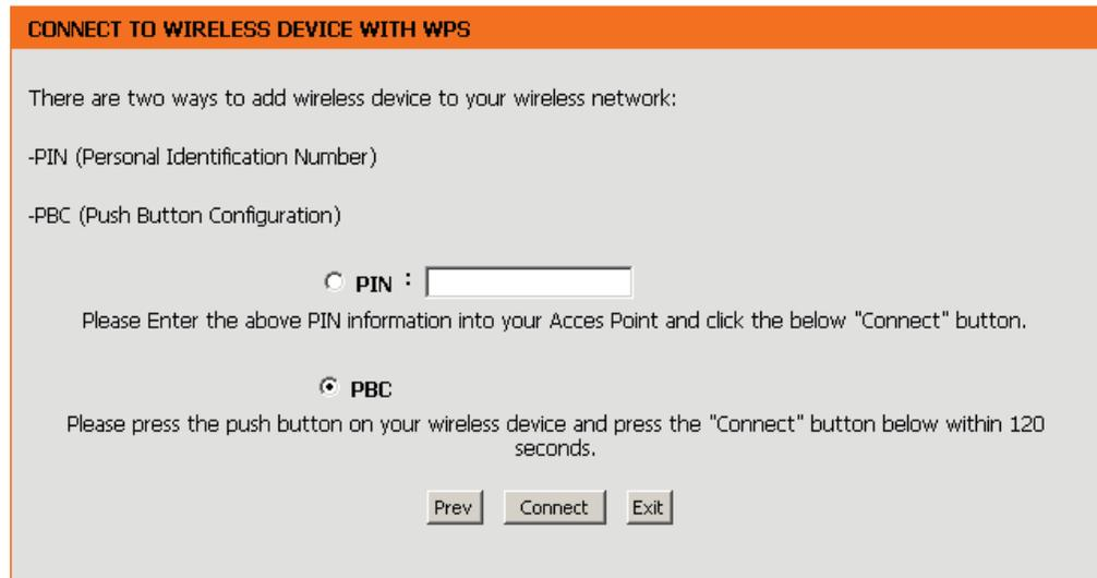
Press down the **Push Button** on the wireless device that you are adding to your network to complete the setup.
