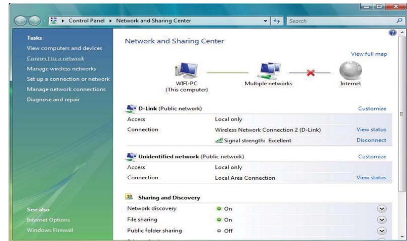
The utility will display any available wireless networks in your area. Click on a network (displayed using the SSID) under Select a network to connect to and then click the **Connect** button.
