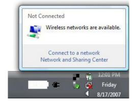
The utility will display any available wireless networks in your area. Click on a network (displayed using the SSID) and click the **Connect** button.
