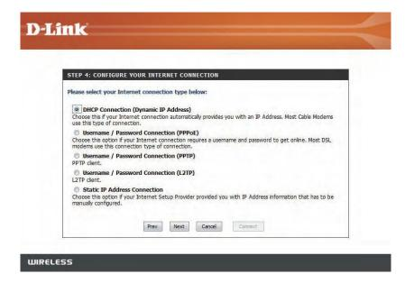
If you selected DHCP Connection, make suer that you are connected to the D-Link router with the PC that was originally connected to your broadband connection. Then, click the Clone MAC button to copy your computer's MAC address. Click Next to continue.
