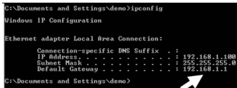
NOTE: If the IP address of Gateway is not displayed, or the address followed by 'IP Address' begins with "169.x.x.x", please recheck network connection between your computer and router, and / or go to the beginning of this chapter, to recheck every step of network setup procedure.
