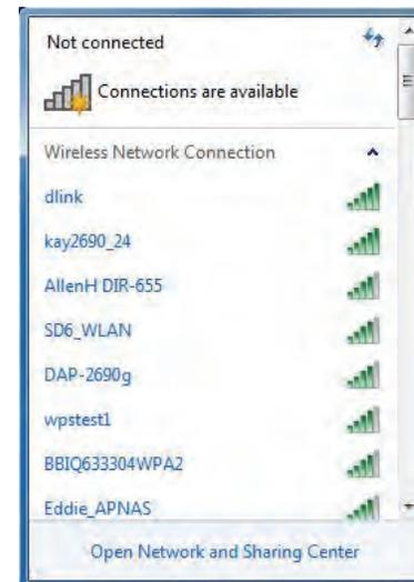
3. Highlight the wireless connection with Wi-Fi name (SSID) you would like to connect to and click the **Connect** button.
