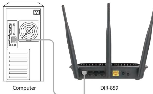
4. Plug one end of the included Ethernet cable that came with your router into the yellow port labeled INTERNET on the back of the router. Plug the other end of this cable into the Ethernet port on your modem.
