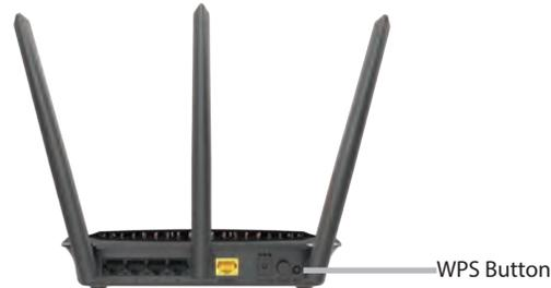
**Step 2** - Within 2 minutes, press the WPS button on your wireless client (or launch the software utility and start the WPS process).
