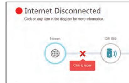
To bring up more details about your Internet connection, click on the **Internet** icon. Click **IPv4** or **IPv6** to see details of the IPv4 connection and IPv6 connection respectively.
