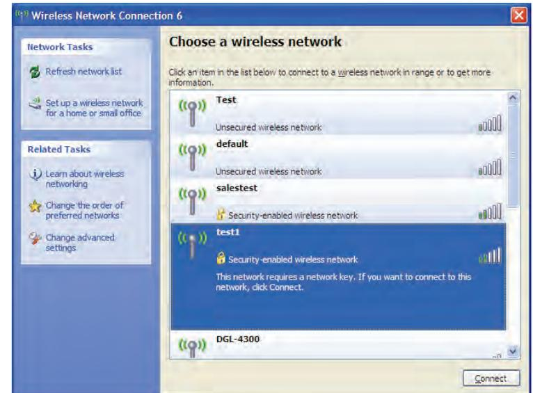
3. The **Wireless Network Connection** box will appear. Enter the WPA-PSK Wi-Fi password and click **Connect**.
