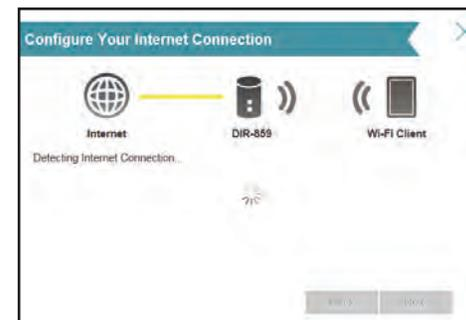
If the router does not detect a valid Internet connection, a list of connection types to choose from will be displayed.
