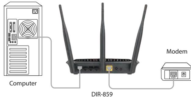
5. Reconnect the power adapter to your cable or DSL broadband modem and wait for two minutes.
