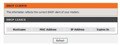
This page displays all client devices that obtain IP addresses from the device. You can view the host name, IP address, MAC address and time expired(s).
