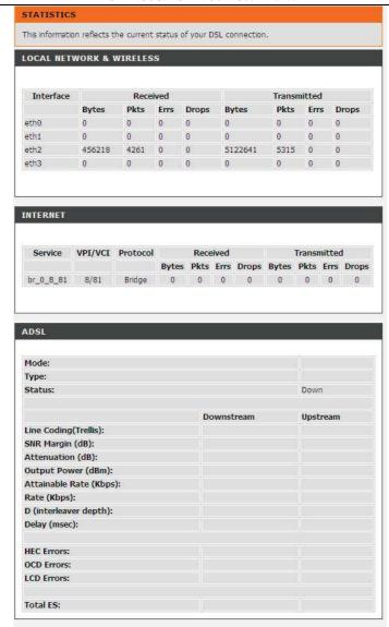
This page displays the statistics of the network and data transfer. This information helps technicians to identify if the device is functioning properly. The information does not affect the function of the device.
