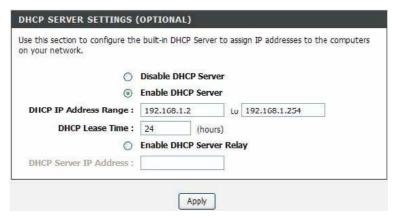
Click **Apply** to save the settings. In the **Local Network** page, you can assign IP addresses on the LAN to specificindividual computers based on their MAC addresses.
