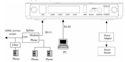
Figure 4 Connection diagram (with a telephone set before the splitter) Connection 1 is recommended.
