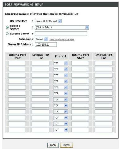
Select a service for a preset application, or enter a name in the **Custom Server**field. Enter an IP address in the **Server IP Address** field, to appoint the correspondingPC to receive forwarded packets. The Ports show the ports that you want to open on the device. The **TCP/UDP**means the protocol type of the opened ports.
