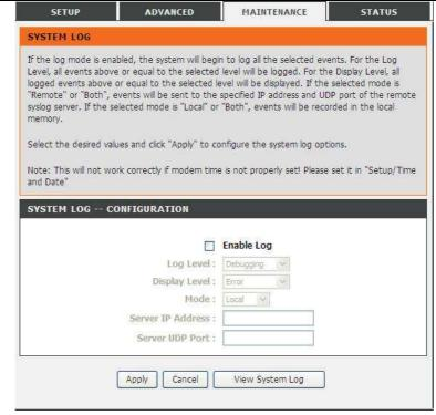
This page displays event log data in the chronological manner. You can read theevent log from the local host or send it to a system log server. Available eventseverity levels are as follows: Emergency, Alert, Critical, Error, Warning, Notice, Informational and Debugging. In this page, you can enable or disable the systemlog function. The procedure for logging the events is as follows:
