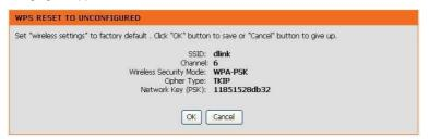
Once the "Reset to Unconfigured" button is clicked, the "wireless settings" will be reset to factory default, other settings will remain unchanged.
