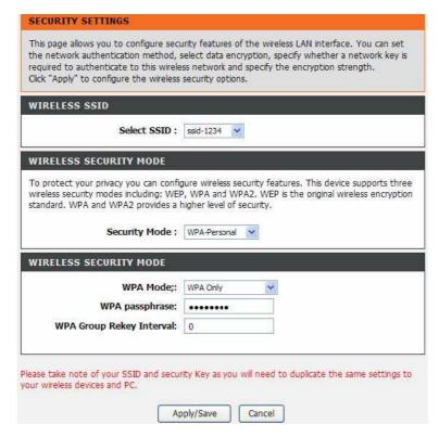
Select the SSID that you want to configure from the drop-down list. Select the encryption type from the **Security Mode** drop-down list. You can select**None**, **WEP**, **WPA-Personal** and **WPA-Enterprise**. If you select **WEP**, the page shown in the following figure appears.
