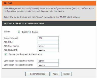
WAN Management Protocol (TR-069) allows a Auto-Configuration Server (ACS)to perform auto-configuration, provision, collection, and diagnostics to this device. In this page, you may configure the parameters such as the ACS URL, ACSpassword, and connection request user name. After finishing setting, click **Apply** to save and apply the settings.
