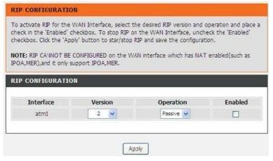
If you are using this device as a RIP-enabled device to communicate with others using the routing information protocol, enable RIP and click **Apply** to save the settings.
