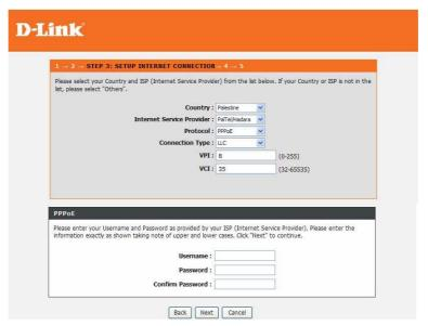
In this page, enter the user name and password. If the Protocol is  $\bf Dynamic\ IP$ , the page shown in the following figure appears.
