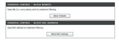
This page provides two useful tools for restricting the Internet access. **Block Websites** allows you to quickly create a list of all websites that you wish to stop users from accessing. **Block MAC Address** allows you to control when clients or PCs connected to the device are allowed to access the Internet.
