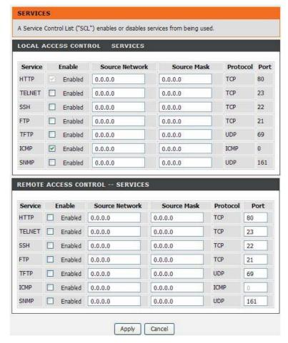
In this page, you can enable or disable the services that are used by the remote host. For example, if telnet service is enabled and port is 23, the remote host can access the device by telnet through port 23. Normally, you need not change the settings. Select the management services that you want to enable or disable on the LAN or WAN interface.
