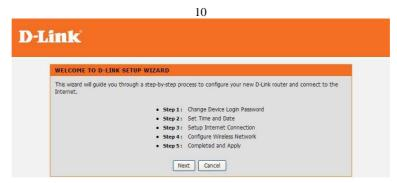
**Step 3** There are four steps to configure the device. Click **Next** to continue. **Step 4** Change Device Login Password. The default password is "admin", in order to secure your network, please modify the password. Note: Confirm Password must be the same as "New Password". Of course, you can click Skip to ignore the step.
