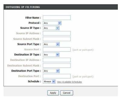
Enter the **Filter Name** and specify at least one of the following criteria: protocol,source/destination IP address, subnet mask, and source/destination port. Click **Apply** to save the settings. The **ACTIVE OUTBOUND IP FILTER** shows detailed information about each created outbound IP filter.
