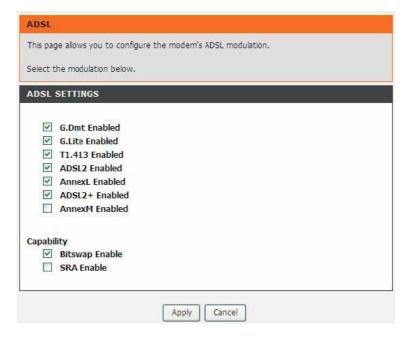
In this page, you can select the DSL modulation. Normally, you can keep the factory default setting. The device negotiates the modulation mode with DSLAM. Click **Apply** to save the settings.
