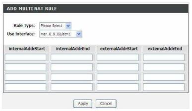
In this page, please select the proper type; select the proper **Use interface**, and configure the other parameters in this page. After finishing setting, click **Apply** to save the settings.
