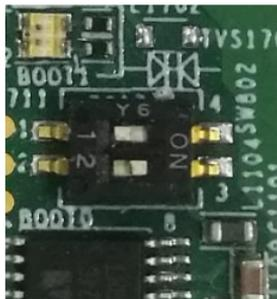
**Figure 4 : SW802 setting for Serial Download Mode**
