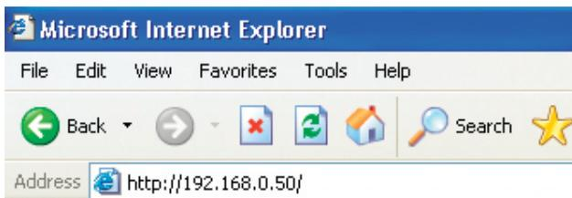
*(The IP Address shown in the example above is the default setting. Use this IP address when connecting to a network consisting of other D-Link devices set to their default settings. If you have changed the IP Address of the DWL-700AP to conform to a network other than one with D-Link devices, then input that IP Address in the web browser, instead of the default IP Address shown.)*
