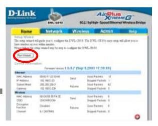
This window displays the default settings of the DWL-G810. The default IP Address is 192.168.30. If you select **Dynamic IP Address**, you will obtain a dynamic IP Address from a DHCP server on your network. The **Subnet Mask** is 255.255.255.0. Input the IP Address of the **Gateway** (the router on your network.) Click **Apply** if you have made any changes.
