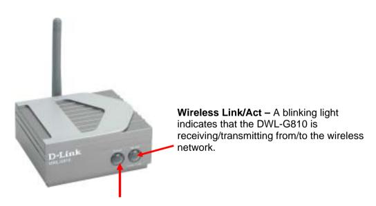
**Power –** a steady **Green** light indicates a proper connection to a power source.
