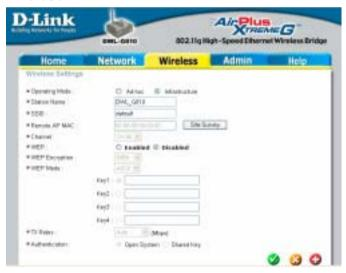
**SSID:** (Service Set Identifier) default is the default setting. The SSID is a unique name that identifies a network. All devices on a network must share the same SSID name in order to communicate on the network. If you choose to change the SSID from the default setting, input your new SSID name in this field. The SSID can be up to 32 characters in length.
