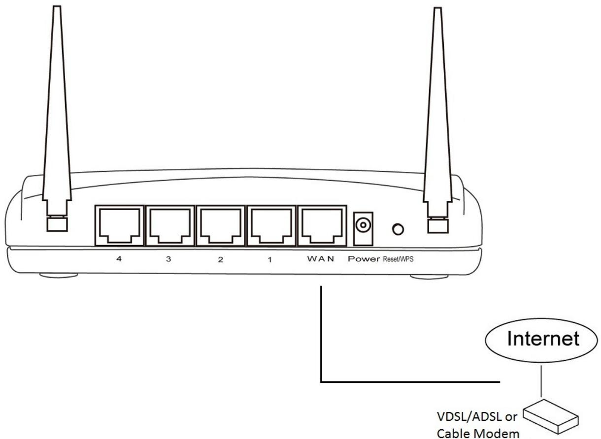
2. Connect all your computers, network devices (network-enabled consumer devices other than computers, like Game console, or Switch / Hub) to the LAN port of the router.
