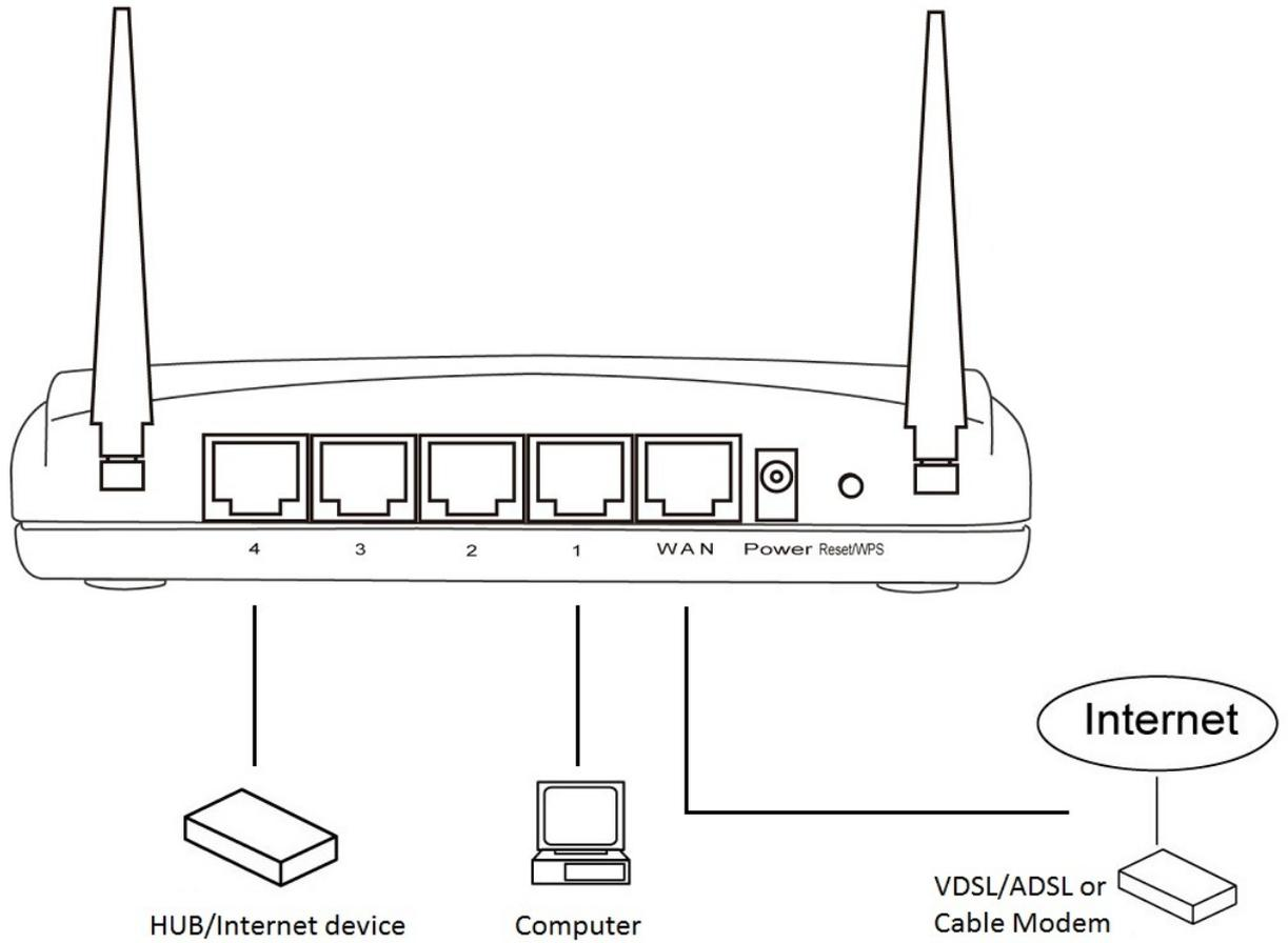
3. Connect the power adapter to the wall outlet, and then connect it to the 'Power jack' of the router.
