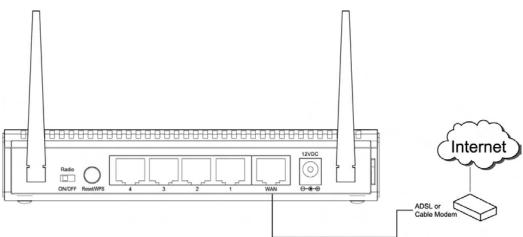
Connect all your computers, network devices (network-enabled consumer devices other than computers, like game console, or switch / hub) to the LAN port of the router.
