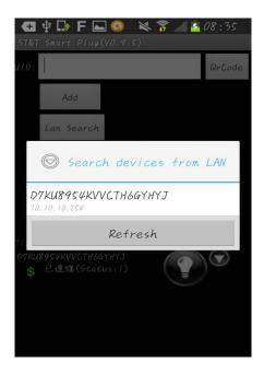
4. Your smart plug will now be displayed on the Smartplug main screen. Slide the switch to switch the your smart plug (and any electrical device you plug into it) on or off.
