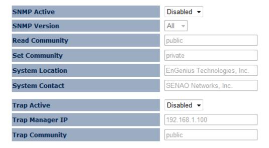
**SNMP Active:** Enable/Disable SNMP function from drop-down list. **SNMP Version:** EOC7510 supports SNMP version v1 and v2c. **Read Community:** Setup the read only community password. **Set Community:** Setup the read and write community password.
