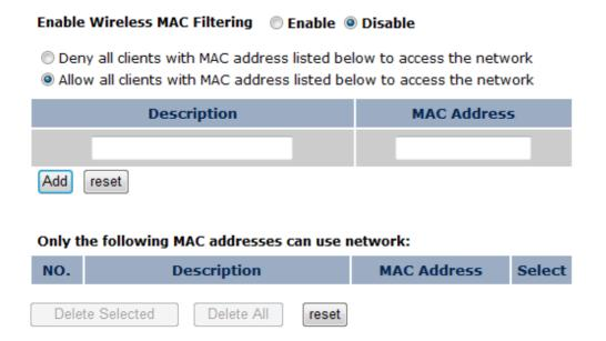
Enable Wireless MAC Filtering: Enable the wireless access control function
