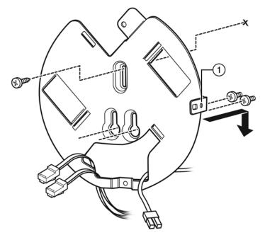
Rivet Hole in Locking Tab
