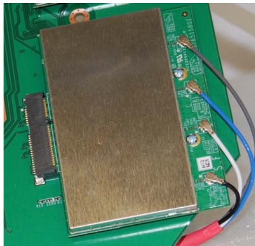
Figure 5 – Connect the Coax Cables to the 802.11ac WiFi Radio Module
