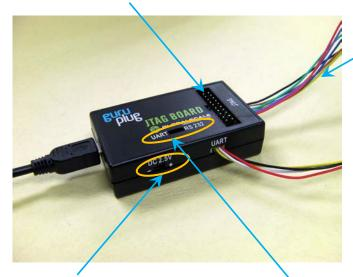
This DC 2.5V is for Dream Plug CPU e-fuse programming only, do not use it for other purpose.
