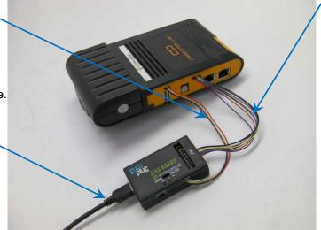
This is the standard 20pin JTAG connector which has the same pin signals as 8 pin cable
