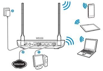
When configuring the WS330 for the first time, use an Ethernet cable to connect the WS330 to a computer.
