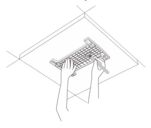
2 Drill holes in the marked positions using hammer drill.
