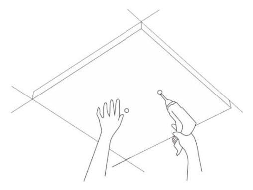
**3** Knock the sleeve anchors into the holes using the rubber hammer.
