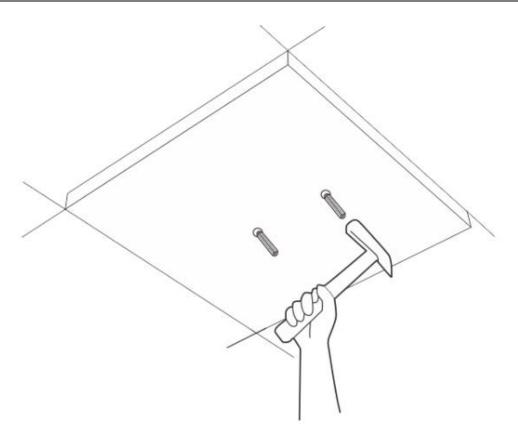
4 Align the screw holes with the holes in the ceiling, and then use the included screws to fix the bracket.
