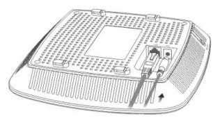
**6** Insert the hooks of the AP into the slots of the bracket, and slide the AP to one side to make sure that the AP is fixed well in the bracket.
