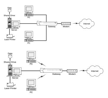
The Intel AnyPoint Networking Gateway 1400 connects directly to a cable modem. Using the gateway and cable modem together enables powerful Internet access on a home or small-business network.
