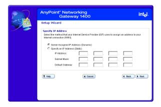
3 Select the Specify an IP Address (Static) option, enter the IP Address, Subnet Mask, and Default Gateway information in the fields provided, then click **Next**.
