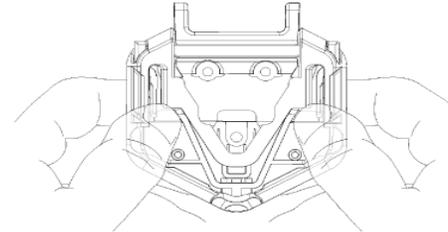
5. If the bracket is closed, open the snaps by pressing in and up with your thumbs on both sides of the snaps on the bottom of the bracket until it is fully open.
