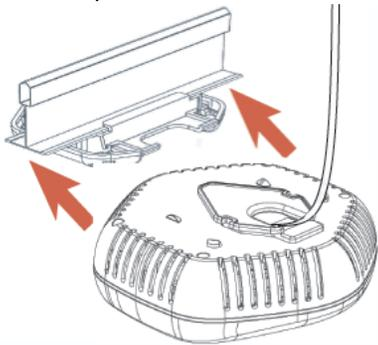
9. If the access point is not properly secured, press the release button on top of the bracket to unlock the access point. Realign the access point, making sure the cable is still connected, and push in on the access point until it clicks securely into place.
