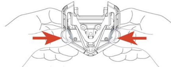
6. With the bracket clips fully extended, align the clips with the rail and hook the clips around the top sides of the rail. Push in on the sides of the bracket until the clips lock over the rail. Listen for a click that indicates that the clips have locked. Be sure the bracket has locked securely onto the rail by gently pulling down on the bracket before installing the access point.
