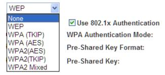
■ WEP —WEP is an encryption scheme that is used to protect user's wireless data communications. WEP uses a combination of 64-bit keys or 128-bit keys to provide access control to user's network and encryption security for every data transmission. To decode a data transmission, each wireless client on the network must use an identical 64-bit or 128-bit key. WEP is an older wireless encryption method that is not as hard to break as the more-recent WPA.
