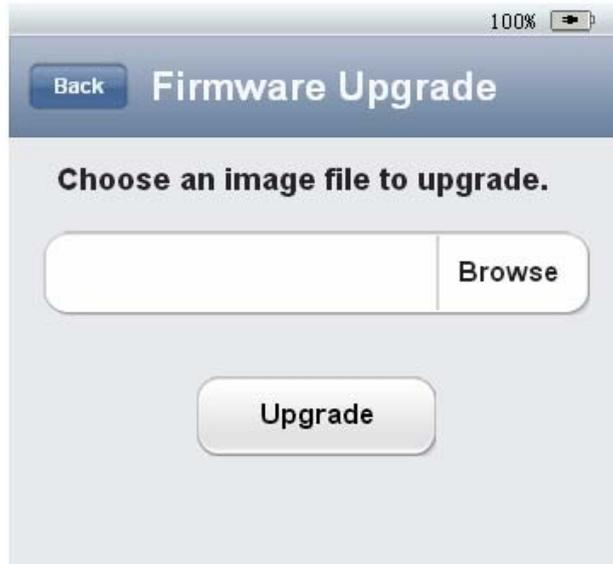
B、Click “System Upgrade” then select “App DB.(Local)” at the drop-down menu of upgrade type , at the same time, there will pop up the following window after selecting “Apply” . The application database needed to be upgraded can be chosen by clicking “Browse”. After clicking “Upgrade” there are 3 minutes waiting to upgrade successfully to appointed Application Database;
