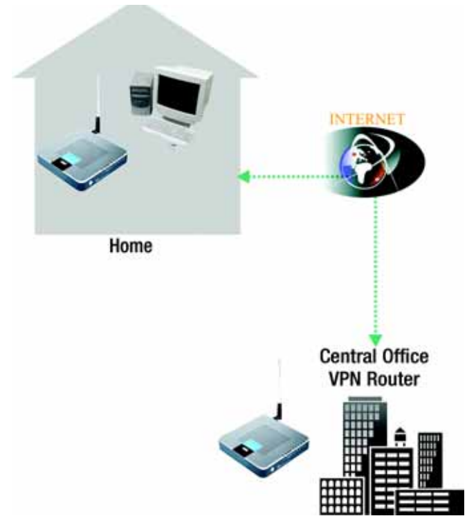
Figure 1-3: VPN Gateway-to-VPN Gateway
