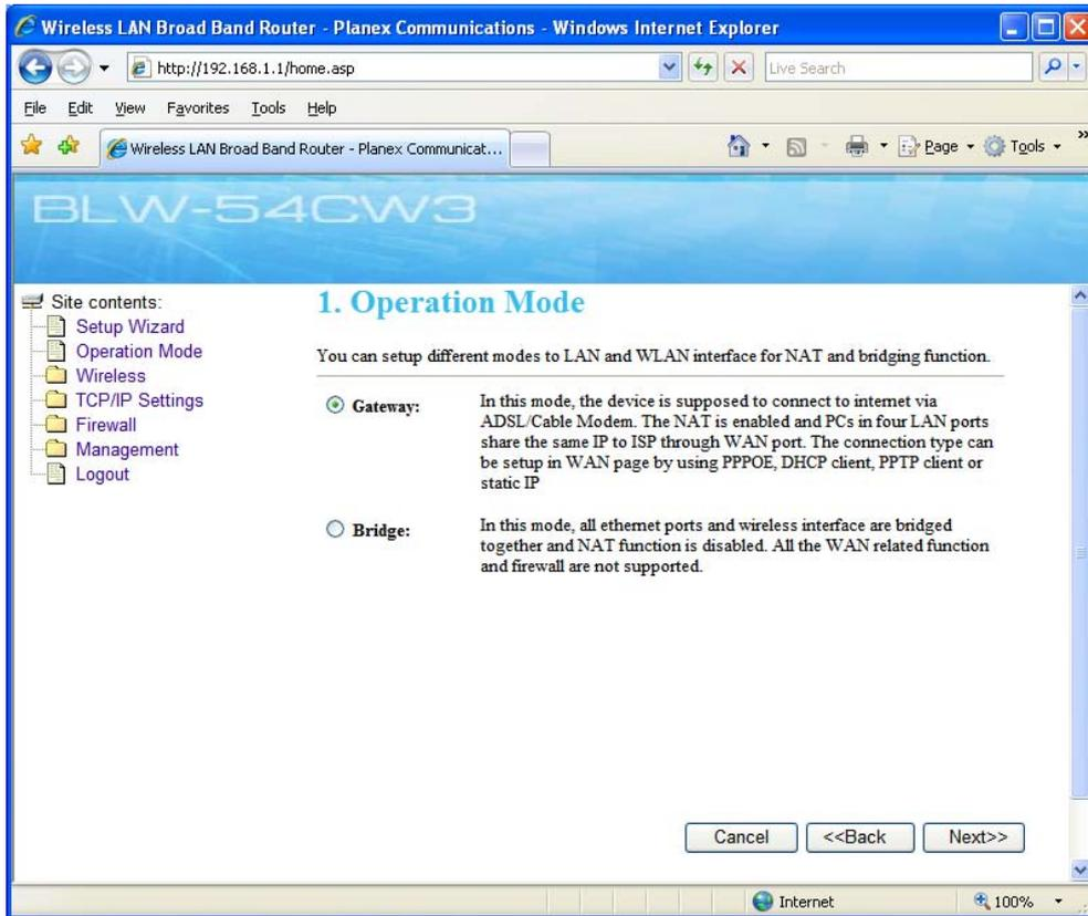
Setup different modes to LAN and WLAN interface for NAT and bridging function. There are two modes that can be chosen: Gateway and Bridge.
