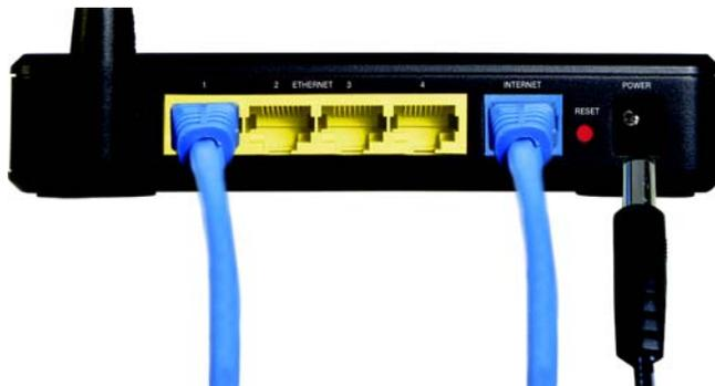
**Figure 4-7: Connecting the Power**
