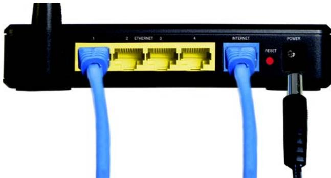
**Figure 4-3: Connecting the Power**
