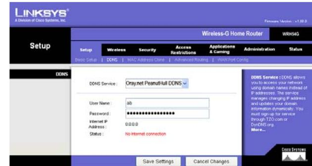
Figure 5-14: Setup Tab - DDNS - Oray.net PeanutHull.com DDNS
