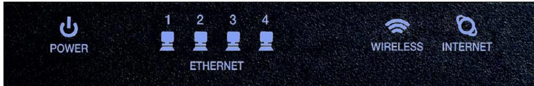
**Figure 3-2: The Router's Front Panel**
