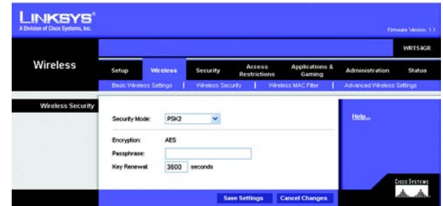
Figure 5-22: Wireless Tab - Wireless Security (PSK2)
