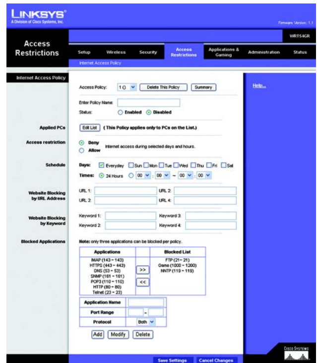
Figure 5-32: Access Restrictions Tab - Internet Access Policy
