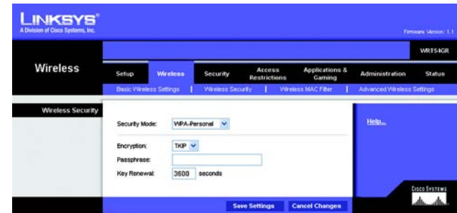
Figure 5-21: Wireless Tab - Wireless Security (WPA-Personal)
