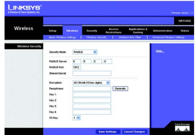
Figure 5-26: Wireless Tab - Wireless Security (RADIUS)
