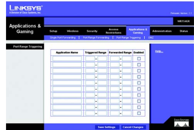
Figure 5-37: Applications and Gaming Tab - Port Triggering
