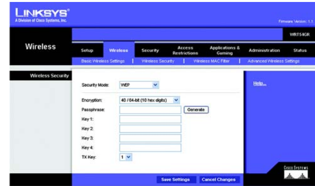
Figure 5-20: Wireless Tab - Wireless Security (WEP)
