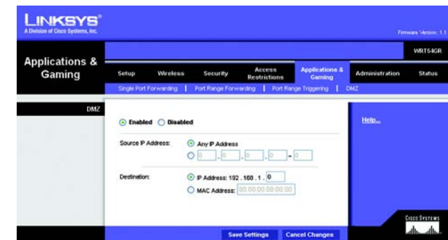
Figure 5-38: Applications and Gaming Tab - DMZ
