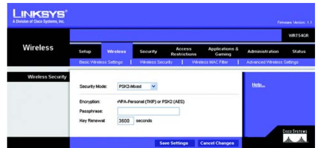
Figure 5-23: Wireless Tab - Wireless Security (RPSK2-Mixed)
