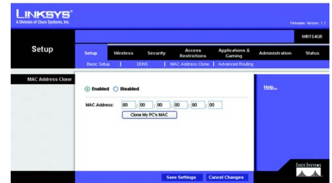
Figure 5-16: Setup Tab - MAC Address Clone
