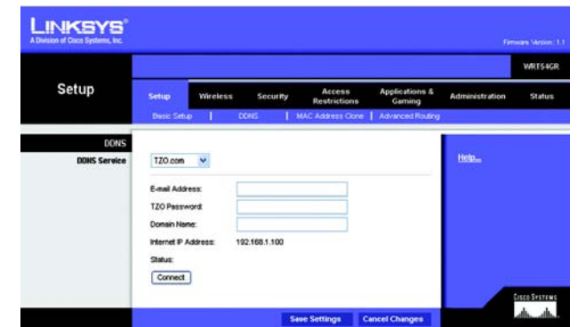
Figure 5-15: Setup Tab - TZO.com
