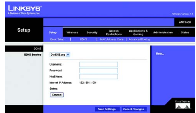
Figure 5-14: Setup Tab - DDNS.com
