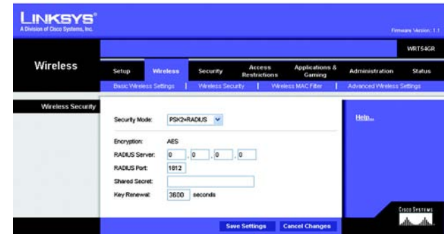
Figure 5-25: Wireless Tab - Wireless Security (PSK2 + RADIUS)
