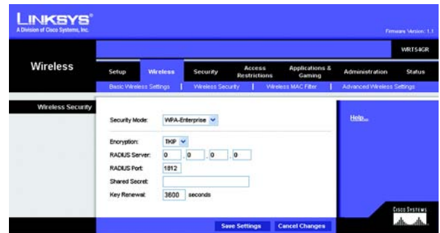
Figure 5-24: Wireless Tab - Wireless Security (WPA Enterprise)
