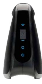
Wireless (Blue) The Wireless LED lights up when there is a wireless connection. The LED flashes when the bridge is actively sending or receiving data over the wireless network.
