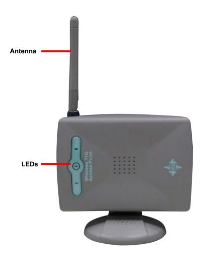
**LEDs** Indicate the power and traffic utilization status.
