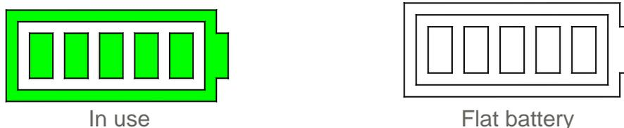
The battery with the lowest remaining charge has the priority and gets connected on the power up. After it is depleted and its indicator turns red the second battery gets connected instead. When both batteries are depleted, with just one red bar remaining they both switch on and continue powering WRN until the power is fully depleted.
