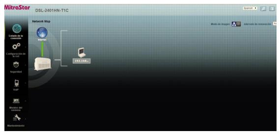
Step 3: Click **Connect to Internet**, Configure the Connection Type and DNS that ISP assigned.
