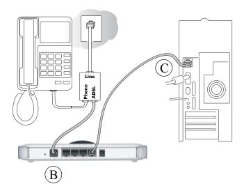
c. Connect the ADSL port (**B**) of the DG834PN to the ADSL connector of the two-line filter.
