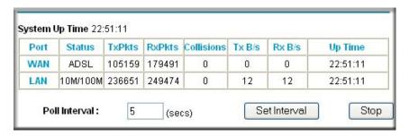
Figure 6-4: Wireless ADSL Modem Router Statistics screen
