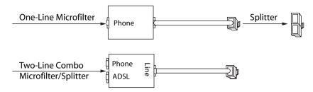
The procedure below illustrates using a two-line combo microfilter/splitter.
