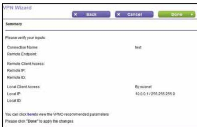
This screen shows the summary of the Wizard configuration with a link to view the VPNC recommended parameters (click **here** to view the VPNC-recommended parameters).
