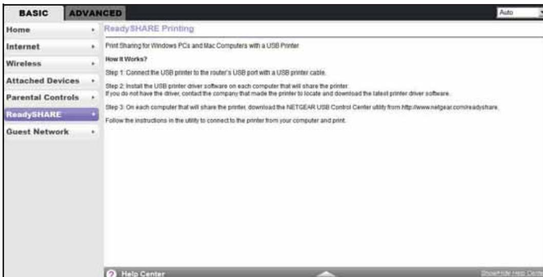
The USB Control Center utility allows you to control a shared USB device from your computer that is connected to the USB port on your router. The utility allows you to control a printer.
