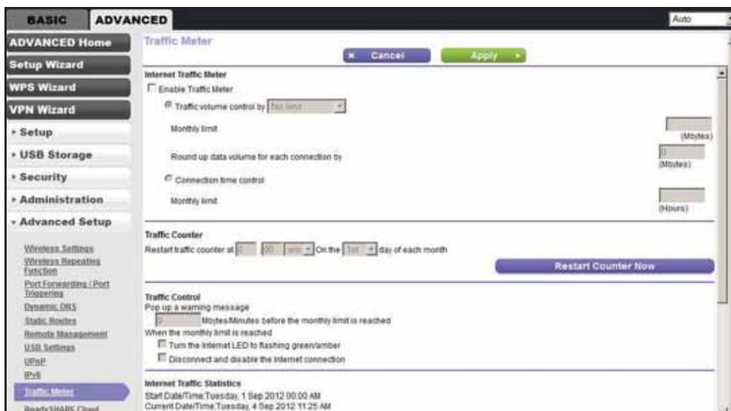
2. To enable the Traffic Meter, select the **Enable Traffic Meter** check box.
