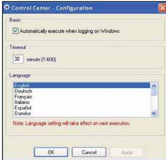
**Automatically execute when logging on Windows.** Select this check box to have the utility start automatically when you are logged in to Windows.
