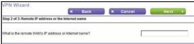
Enter the remote IP address of the Gateway you want to connect to, or provide the Internet name of the Gateway. The Internet name is the Fully Qualified Domain Name, as setup in a Dynamic DNS service.
