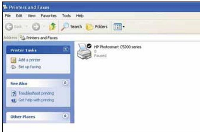
This USB printer is ready. The utility does not need to always hold the connection of this USB printer. Once there is any print job for this printer, the USB utility connects to this USB printer automatically, then prints. After the print job is done, the printer status returns to the Paused state.
