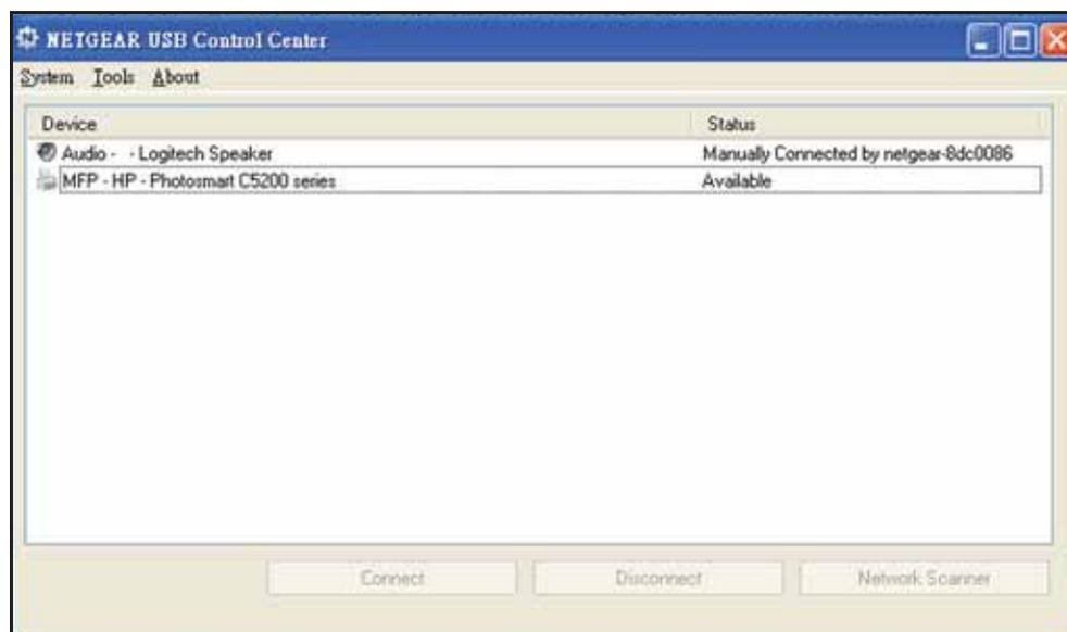
This screen is the main screen, which shows a device icon, the description for this USB device, and its status.
