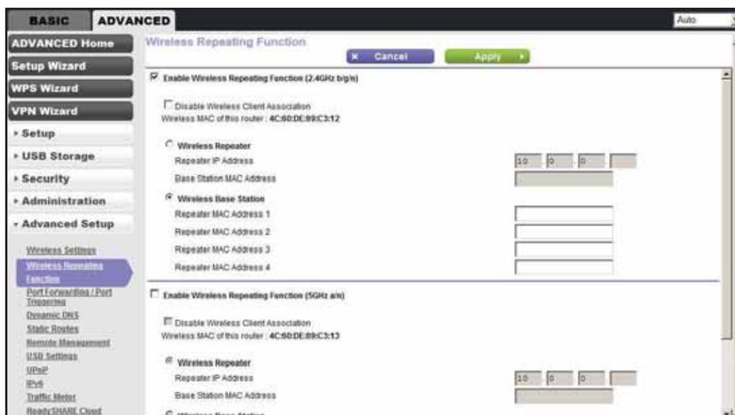
3. In the Wireless Repeating Function screen (depending on the frequency you want to use), select the **Enable Wireless Repeating Function** check box and select the **Wireless Base Station** radio button.
