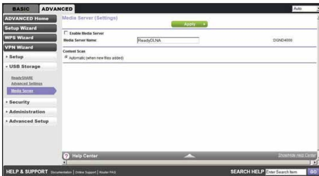
By default the Enable Media Server check box and the Automatic (when new files are added) radio button are selected. When these options are selected, the wireless modem router scans for media files whenever new files are added to the ReadySHARE USB hard drive.
