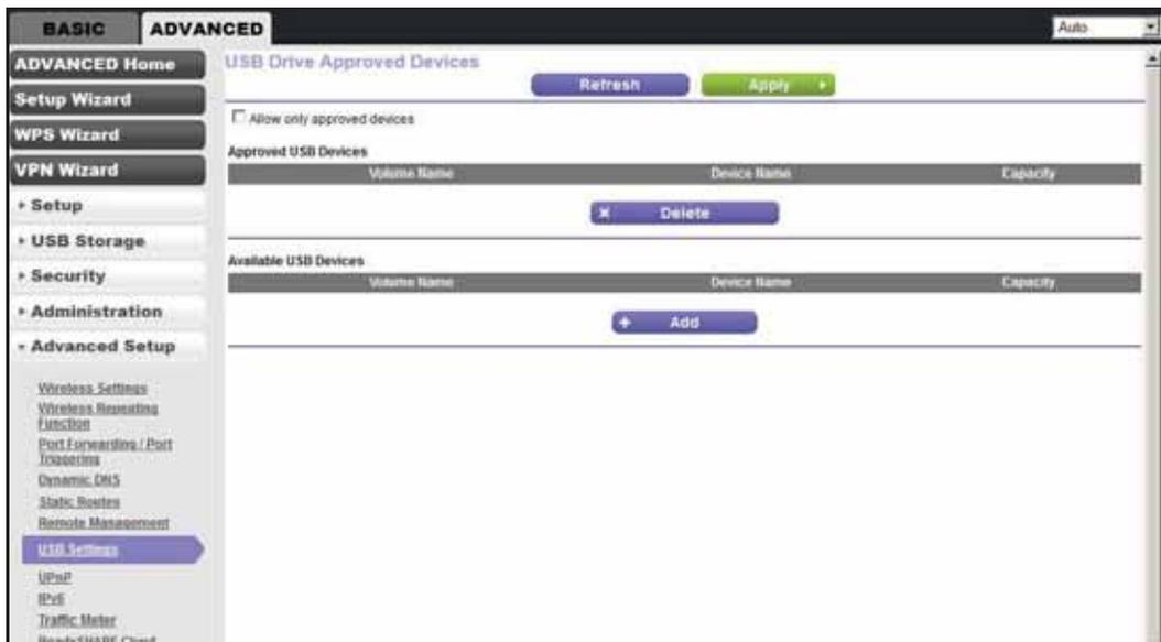
This screen shows the approved USB devices and the available USB devices. You can remove or add approved USB devices.
