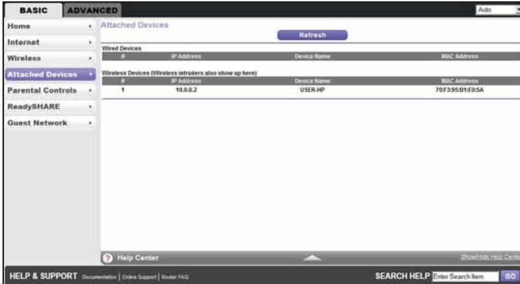
Wired devices are connected to the wireless modem router with Ethernet cables. Wireless devices have joined the wireless network.
