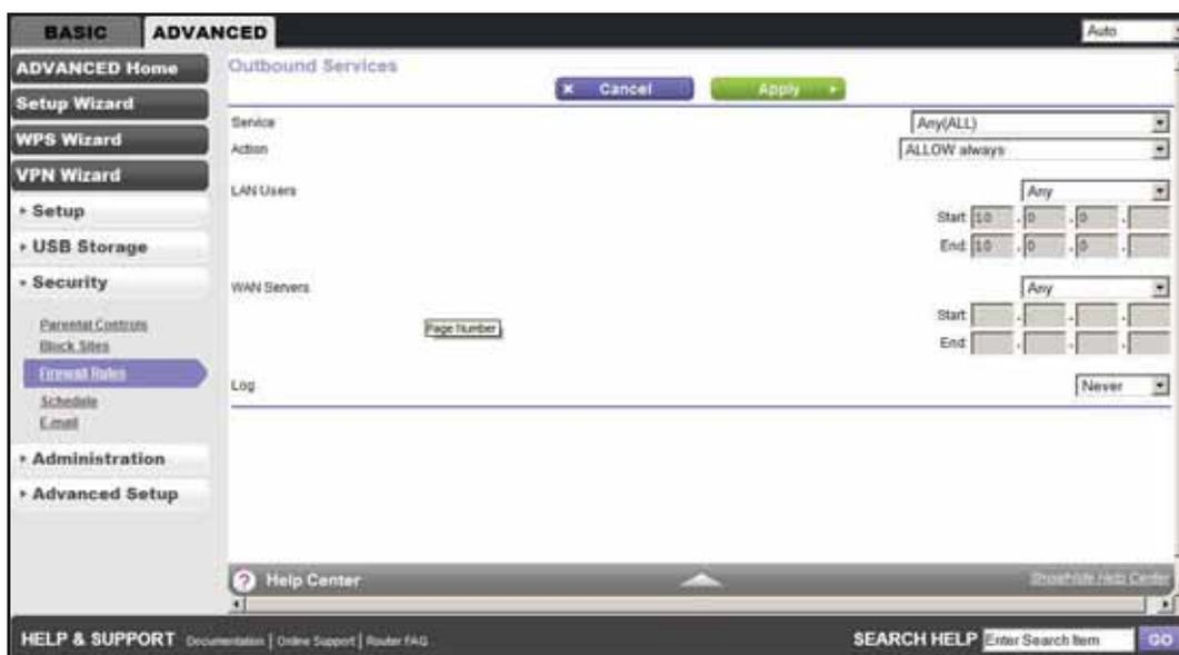
Use the Outbound Services screen to define a new Outbound Firewall rule, or edit an existing rule. The outbound firewall rules are used to block or allow access by computers on your network to services or applications on the Internet.
