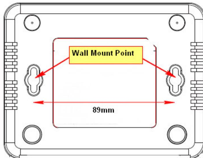
You can mount the device on the wall. There are two mounting points on the bottom of the device. Please find a proper spot where two nails can be applied. The distance between the two nails is 89mm. Finally, carefully mount the device onto the wall and make sure the nails are firmly locked on the mount points.
